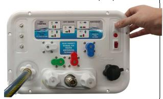
**NOTE**: LED indicator light below the pump switch will be lit if pump has power.
