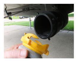
2. Open black waste holding tank valve and leave open to allow black tank to drain.
