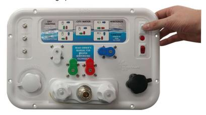
3. Push "PUMP" switch to turn pump on.
