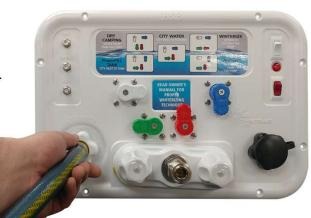
3. Place other end of hose in container holding water or sanitizing solution.
